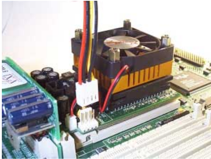
Figure 6. Connecting the power cable
