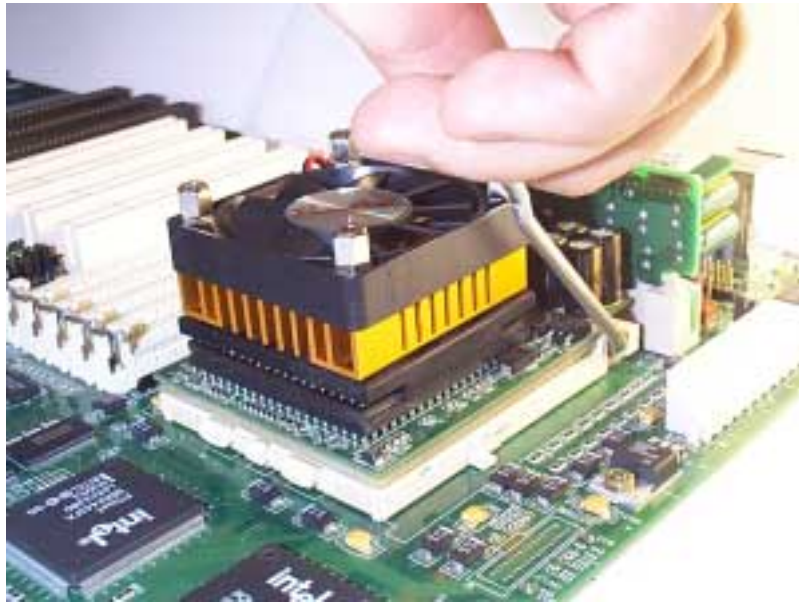
Figure 5. Locking the upgrade adapter into the ZIF socket
