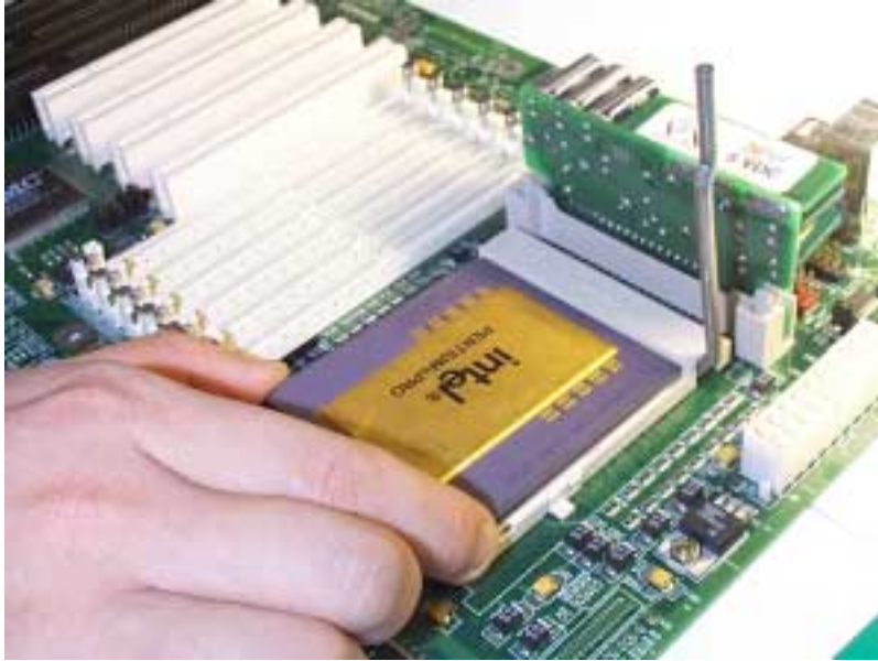
Figure 3. Removing the Pentium Pro CPU
