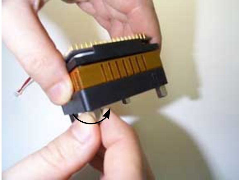
Figure 2. Tightening the hex nuts
